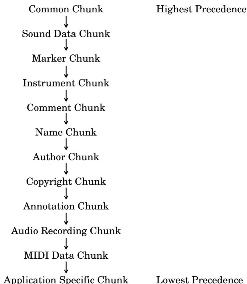
The *Common Chunk* has the highest precedence, while the *Application Specific Chunk* has the lowest. Information in the *Common Chunk* always takes precedence over conflicting information in any other chunk. The *Application Specific Chunk* always loses in conflicts with other chunks. By looking at the chunk hierarchy, for example, one sees that the loop points in the *Instrument Chunk* take precedence over conflicting loop points found in the *MIDI Data Chunk*.
