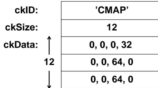
The fixed header part means "Here's a type ckID chunk with ckSize bytes of data."
