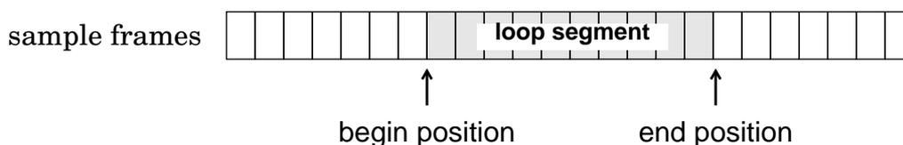
With forward/backward looping, the loop segment is first played from the begin position to the end position, and then played backwards from the end position back to the begin position. This flip-flop pattern is repeated over and over again until interrupted.
