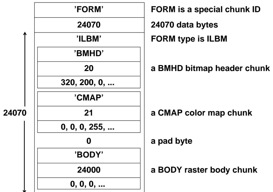
A FORM always contains one 4-character FORM type ID (a file type, in this case 'ILBM') followed by any number of data chunks. In this example, the FORM type is 'ILBM', which stands for "InterLeaved BitMap". ILBM is an IFF standard for bitplane raster pictures. The bitplanes are interleaved so you can process a scan line at a time. This example has 3 chunks. Note the pad byte after the odd length chunk.
