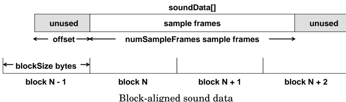
In the above figure, the first sample frame starts at the beginning of block N. This is accomplished by skipping the first `offset` bytes of the `soundData`. Note too that the `soundData` array can extend beyond valid sample frames, allowing the `soundData` array to end on a block boundary.
