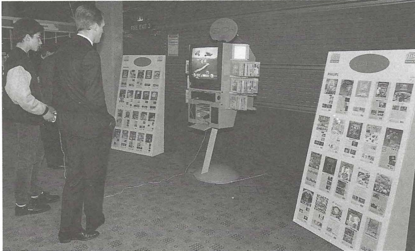
The UK's CD-I kiosk enables display and demonstration of the system in retail outlets. Software titles are displayed on racks at the sides.
